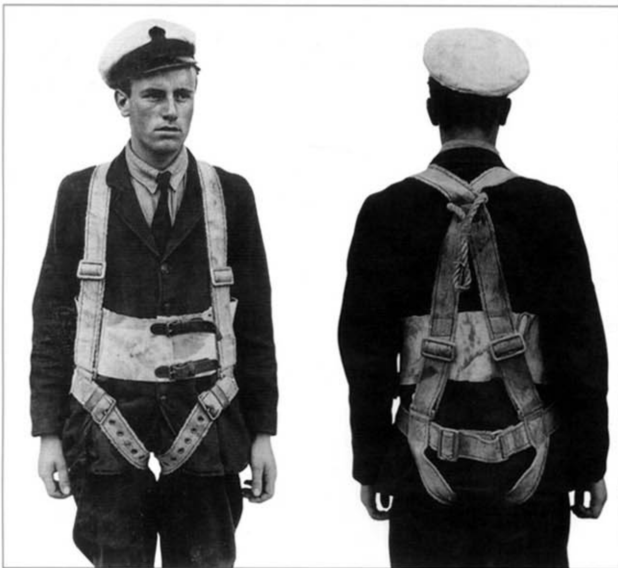
One of the more sophisticated designs of parachute harness, permitting easy adjustment of the strap lengths to ensure a comfortable fit. The suspension point from between the shoulders permits no chance of control during the descent, however. (RAFM P015842 & 3)
