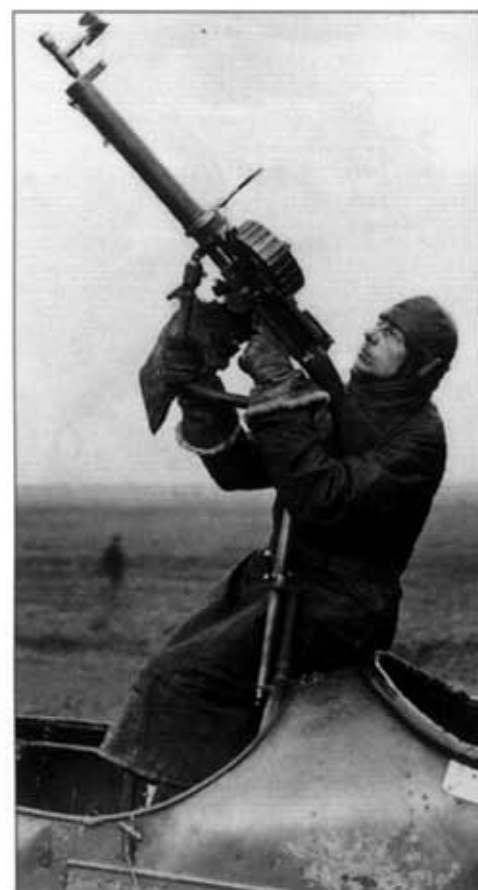
Although a posed ground shot this picture shows the terribly exposed position, both to slipstream and enemy fire, of an FE2 gunner using the rear gun mounting. The front mounting gave no more cover. No safety harness was available until very late in the war. (RAFM P4800)
