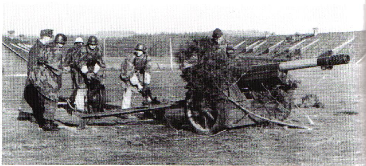
A section of Artillerie-Regiment 22 training at Fallingbommel in February 1943. Wearing the Zeltbahn as an outer garment, this crew operates a 75 mm Pak 97/38—a French 7.5 cm model 1897 gun modified with the carriage of the German 5 cm Pak 38. This weapon formed the backbone of the artillery for most LwFD.
