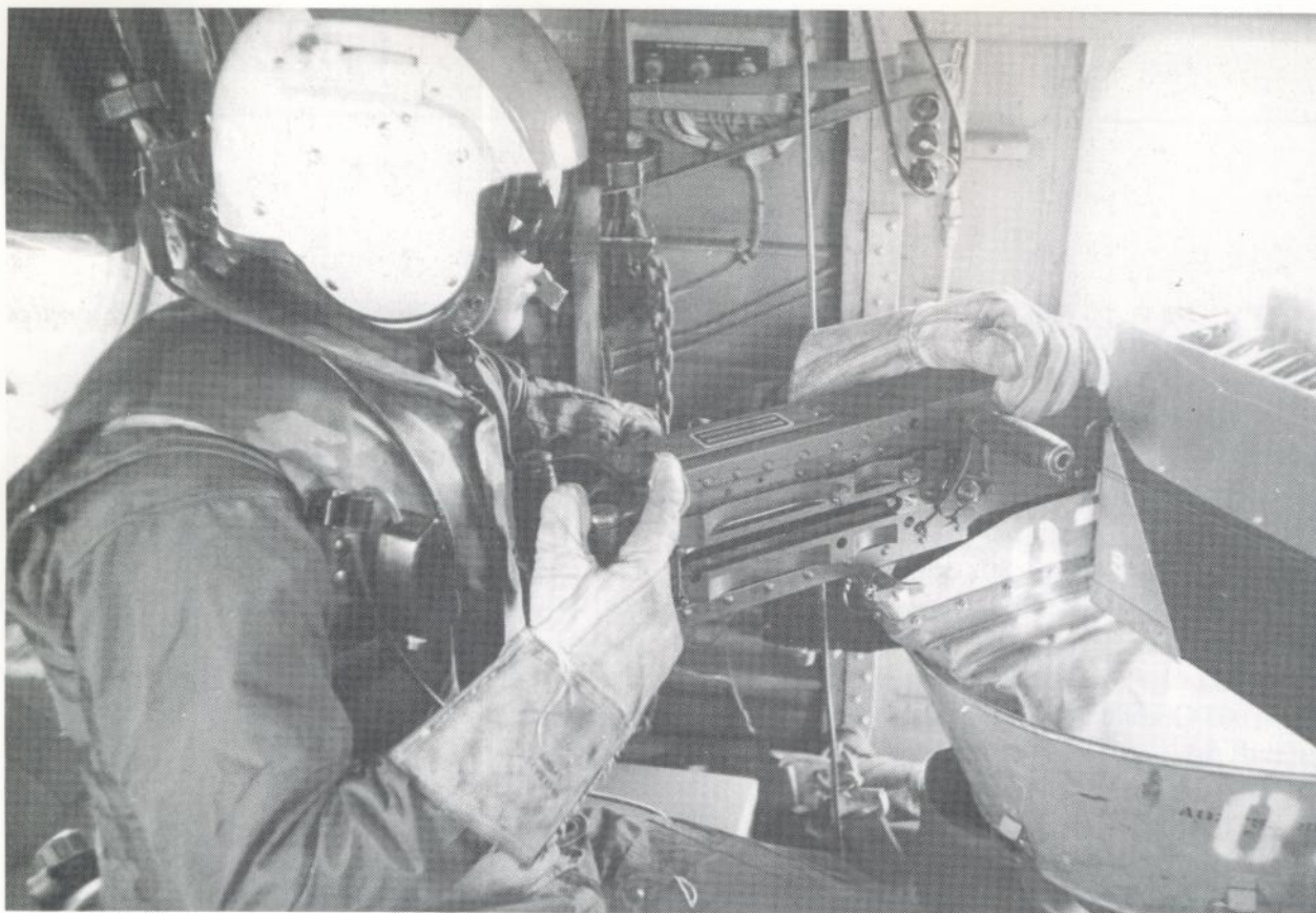
Marine helicopter crewman mans a .50cal. Browning MG from the gunner's position of a CH-46D Sea Knight . He wears the Navy/Marine Corps SPH-3B helmet, PASGT body armour and standard CWU-27 flight suit. The heavy canvas gauntlets facilitate changing hot barrels, clearing jams, etc. (US Marine Corps)
