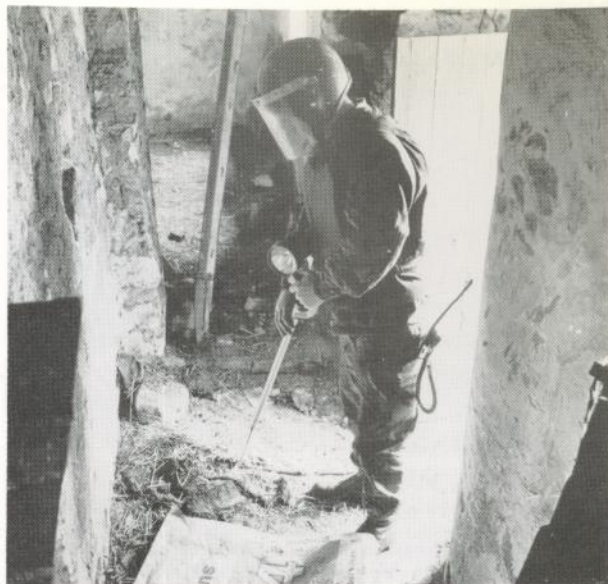
A member of a Royal Engineer Search Team uses his No. 6 Mine Prod to scrutinise an empty bag of fertilizer—one of the constituents of IRA 'Co-op mix' bombs—in a farm outhouse near the Irish border. He is wearing 'US Variable Body Armour' with ceramic plates, front and rear, and an ART helmet. Search teams now use a range of purpose-designed body armour items, including a special helmet incorporating communications equipment. ( Soldier Magazine )
