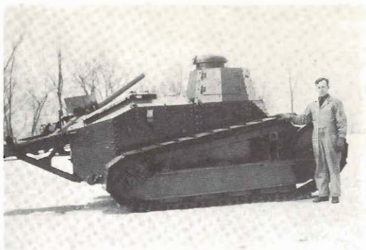
A French-made Renault light tank, with a crew of two and very slow speed, was the mainstay of American armour. George S. Patton, Jr., made his reputation as an armour commander during World War I.
