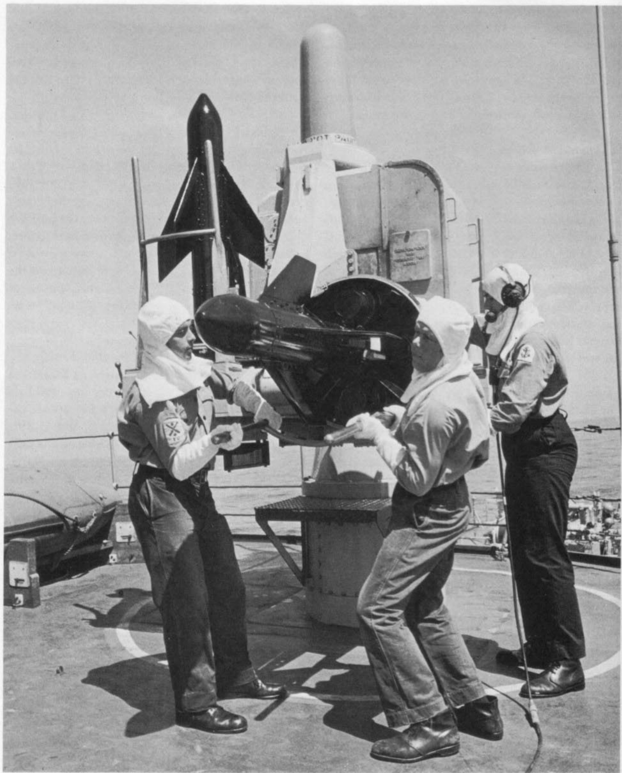
39. Ratings loading a Seacat missile launcher on board HMS Hermione . Working dress now consists of blue shirts with relevant rank patches on the sleeves and name tallies above the left pocket; blue denim or serge trousers with canvas belts; and black boots or plimsolls. Note anti-flash gloves and hoods. (Crown Copyright)
