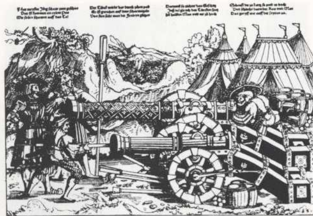
Medium artillery pieces, probably Kartaunen. In general the rate of firing was slow. This was in part due to the necessity to cool and clean the bore each time to prevent premature explosions when reloading; vinegar was used to cool the barrels.
