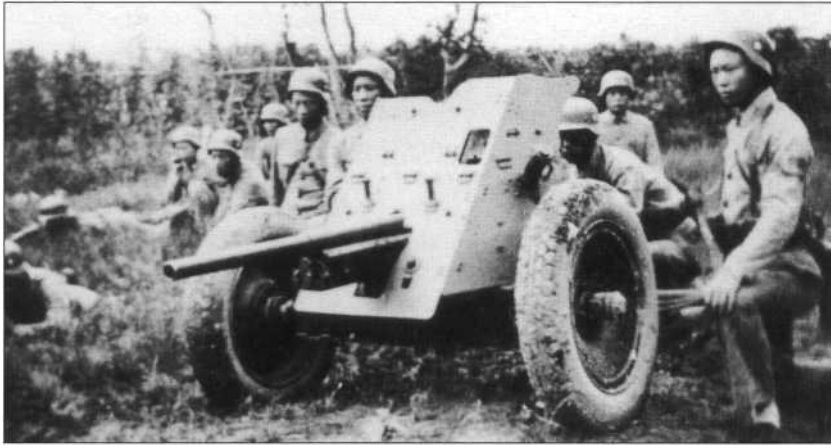
The Chinese Army in general was pitifully short of modern heavy weapons, and any modern equipment was invariably given to the units most loyal to Chiang Kai-shek. This 3.7cm German Pak 36 anti-tank gun was photographed in 1937, when it could still offer a useful defence against Japan's obsolescent tanks. (Joseph T.C.Liu)
