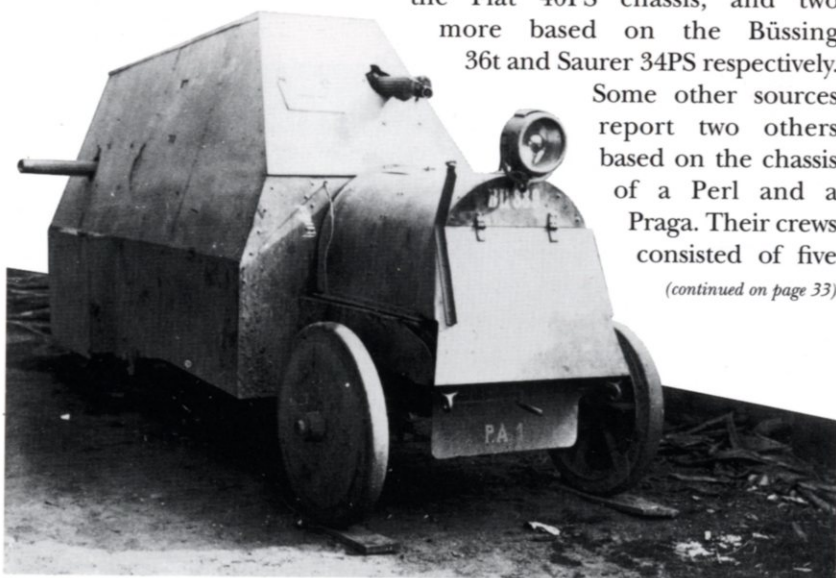
A Junovicz armoured car photographed in Bukovina, armed with three Schwarzlose 07/12 machine guns and carrying a crew of five. 'P.A.1' probably stands for Panzerauto 1 - 'Armoured Car No.1'. Only about half-a-dozen were built, but photos prove that at least one of them saw action during counter-attacks in this region. (Kriegsarchiv)
