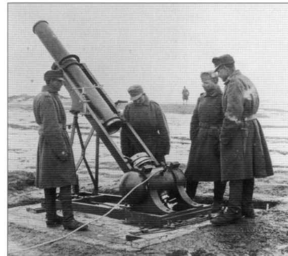
A 20cm Luftminenwerfer on the Eastern Front in Galicia. This Spitz-Bartelmus system heavy trench mortar, powered by air compressed at 55 atmospheres, could throw bombs - of either 22.5kg (50lbs) or 34.5kg (76lbs) weight - out to about 1150 metres. It weighed 725kg (1,600lbs) and was operated by a crew of five. The compressed air canister had to be replaced for each shot, and the rate of fire was only about ten rounds an hour - its main drawback. (Kriegsarchiv)
