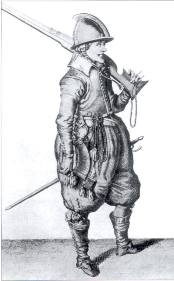
Dutch soldier, early 17th century, armed with a caliver, the light version (about 3.8kg, 8.5lbs) of the matchlock musket; this had a caliber of 20mm (0.75in) and a maximum range of about 200 yards, though it was not accurate at a quarter that distance. Note the cabasset helmet – several have been found at early colonial sites in North America. (Print after De Gheyn)
