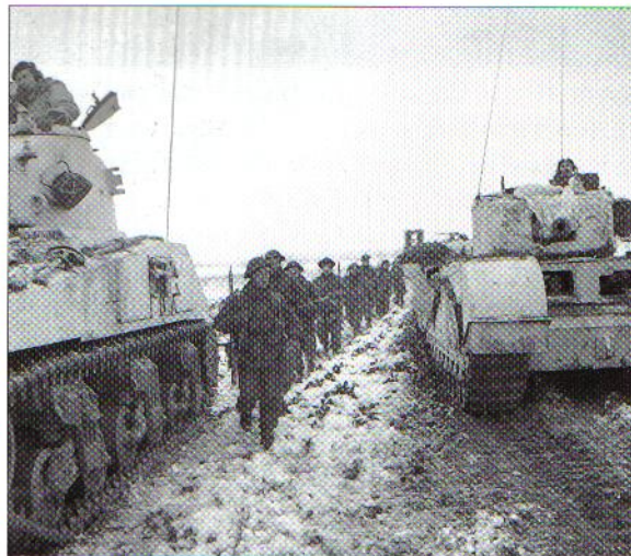
Germany, January 1945: men of C Coy, 4/5th Royal Scots Fusiliers from 156th Bde, 52nd Div, advance past a Sherman and a Churchill tank, both of which have received a coat of whitewash as camouflage. The slow, heavily armoured Churchill was used by non-divisional independent tank brigades for infantry support work. It also provided the basis for various specialist AFVs of 79th Arm Div, including the fearsome Crocodile flamethrower tank. (IWM B13788)
