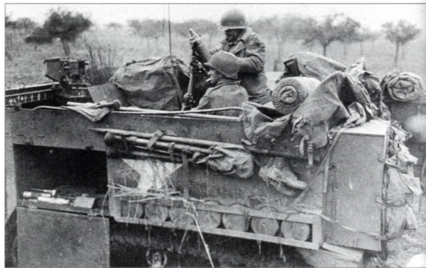
France, 1944: M2 halftrack from an Armored Division mounting an 81mm mortar; and note at left the 'roller coaster' rail for mounting machine guns. This is a good example of the 'gypsy caravan' look which US vehicles tended to acquire during a campaign of movement.
