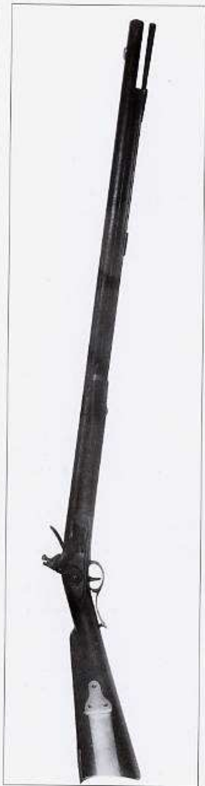
Model 1803 Rifle (Type II) as manufactured at the Harpers Ferry Armory in 1814 to arm the newly-raised rifle corps, although this particular example is of post-war production. It differed only slightly from the original model, e.g. in having its barrel finished bright instead of browned, and having an improved ramrod. (Courtesy William Gavin Collection)
