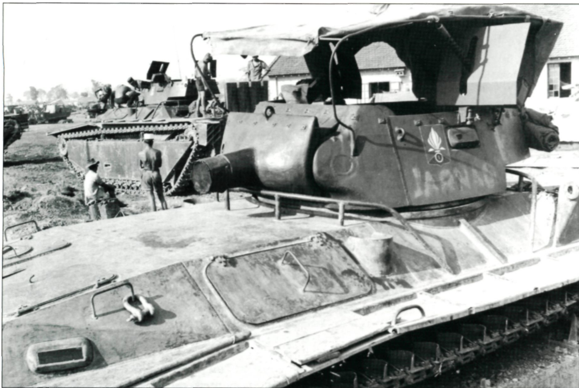
Tonkin, 1954: LVT-A4 amphibious fire support vehicle of the 1 er REC's 2 o GA, fitted with the 75mm howitzer turret from the M8 HMC. By now the 2 o GA had three squadrons (one non-Legion) each with 33 'Crabs'; three squadrons each with eleven LVT-4 'Alligators' carrying Vietnamese infantry; and six LVT-A4s. (ECPA)
