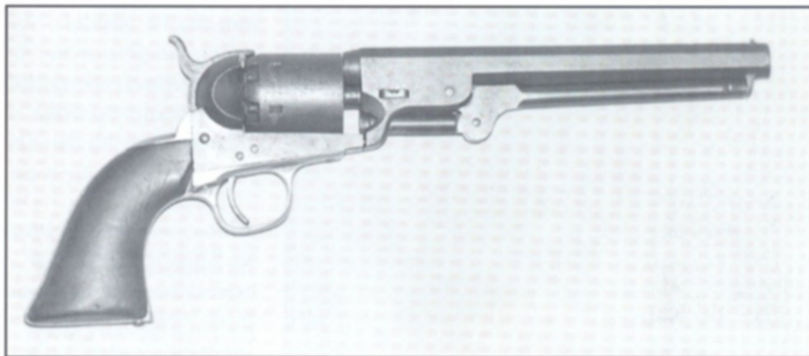
The Model 1851 Colt 'Navy' fired a .36 calibre projectile and provided six rounds when the trooper had to engage the enemy at close range. (Greg Harmon Collection)
