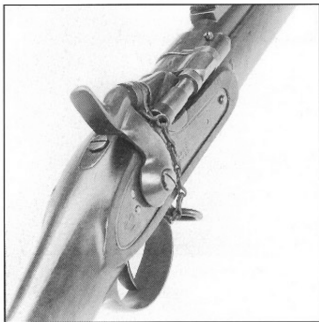
Detail of the lock of an 1862 British Snider rifle supplied to the Turkish army. The breach opened sideways, as did that of the Russian Krnk rifle, but the Snider was the better
