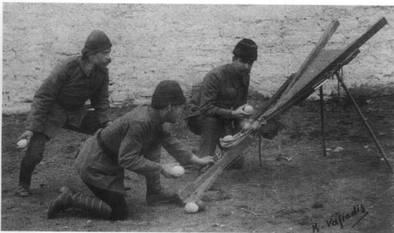
NCOs training with a large wooden grenade-throwing catapult. Naval as well as Army personnel appear in another photograph taken at the same time, indicating that part of the Ottoman Navy was involved in coastal defence. (Askeri Müzesi, Istanbul)
