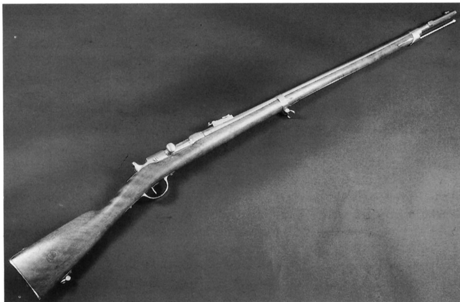
The Chassepot, probably the best rifle then in service in Europe; it far outclassed the Prussian Dreyse needle-gun. Sighted to 1,200 metres and comparatively light, it proved very popular with the troops. (Private Collection)
