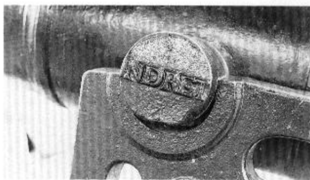
The left trunnion of this M. 1779 naval 18-pdr. gun shows that it was cast at Indret, the main centre for the manufacture of French naval ordnance. From a gun captured from a French ship during the Napoleonic wars and now in Plymouth, Montserrat. (Author)
