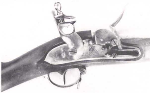
Lock of the 'new' Prussian musket of 1809, as manufactured at Neisse in Upper Silesia. Note the shield around the pan, protecting the priming from the weather, and the firer's face from the flare of the priming.
