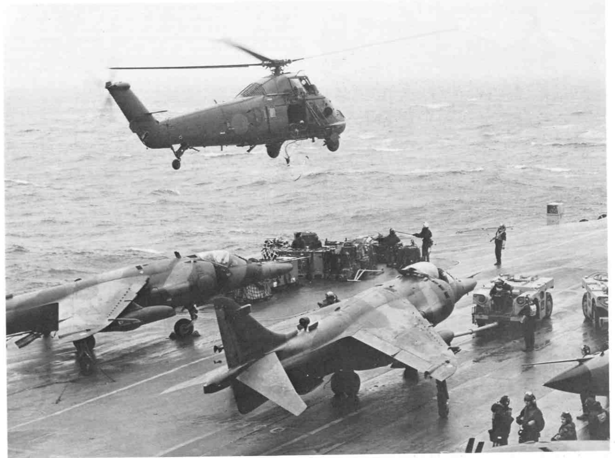
Wessex HU.5 hovering above two Harrier GR.3s on Hermes . It is interesting to note that the camouflage pattern has been hastily extended to cover the upper wing roundels. (MoD)
