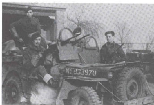
Rhodesian members of the British SAS regiments pose with a jeep modified for use by SAS in NW Europe. The front seats and twin Vickers K gun mount are armoured and have armour-glass windshields. A Bren is mounted on the wing beside the driver. The gunner wears a maroon beret; a Denison smock; despatch rider's boots with turned-down socks and a commando knife stuck in the top; and a holstered pistol slung low on the hip. Tank driver's gauntlets are worn by two of this group. (SAS Regt. Assoc.)
