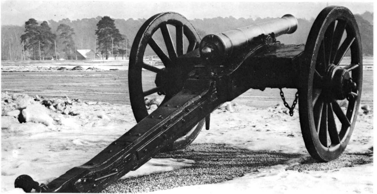
British 9pdr. brass gun on Congreve block trail carriage. Note axle boxes. (National Army Museum)
