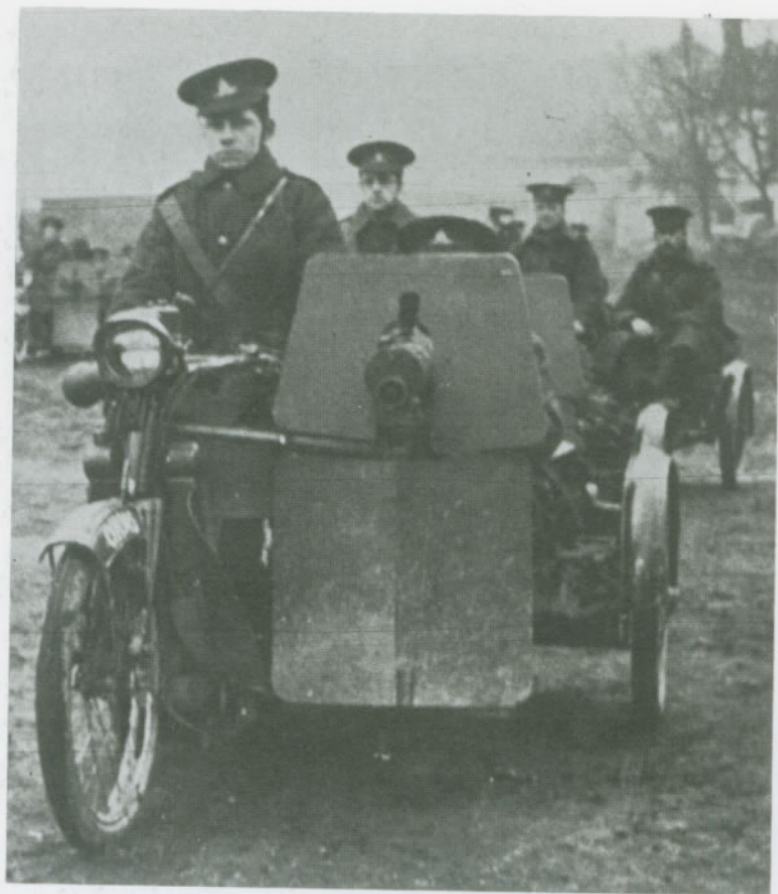
Clyno/Vickers motorcycle and machine gun combination, typical of various combinations used from 1914 onwards in support of, or in place of, mounted cavalry; as the war progressed they were used more and more as machine gun carriers. The gun was not intended to be fired from the sidecar, but from the normal tripod mount which was stowed behind the seat. By 1918 there were some 1,800 Clyno/Vickers combinations in service.
