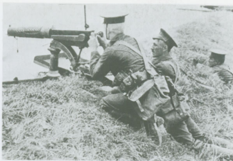
Maxim gun crew, 1914; at this time every infantry unit had a section of two guns served by an officer and twelve men, mostly expert marksmen. For each gun 3,500 rounds were carried, with another 8,000 in reserve. The Maxim and carriage weighed approx. 9½cwt, and fired 500rpm. Late in 1915 it was gradually replaced by the Vickers, weighing 40lbs and firing 500rpm. After the formation of the Machine Gun Corps during the war infantry and cavalry units received increased firepower with the issue of the Lewis LMG, weighing 28½lbs and fed from 47-round drums. This was air-cooled, with an outer casing of aluminium and a radiator.
