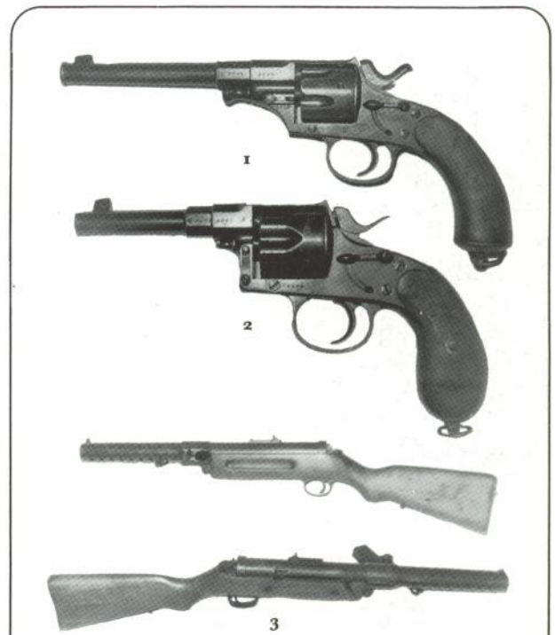
Three of the least well-known weapons used by the German Army during World War I: (1) The Reichs Revolver M/79 Cavalry Model, issued to artillery drivers and reserve units; calibre 10.55mm. (2) The Reichs Revolver M/79 Infantry Officers' Model, and issued to reserve units; 10.55mm calibre. (3) The MP (Machinepistole) 18 I Bergmann; 9mm calibre, weighing 4kg. Introduced during the summer of 1918 on the Western Front and used mainly by special formations and assault troops. It had a drum magazine holding 32 rounds and was issued to all officers, NCOs, and ten men from each assault company. In infantry companies it was issued to 6 men who formed a 'Machinepistole Truppe'. (Imperial War Museum)
