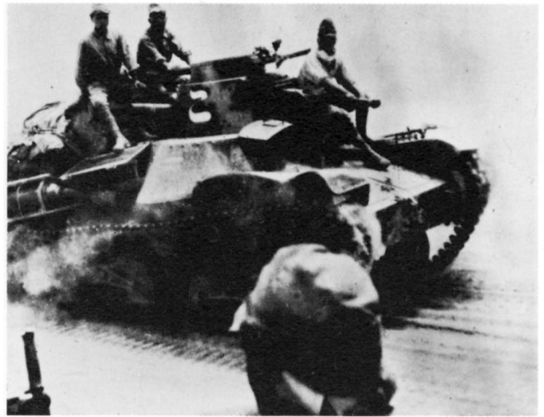
The Japanese made no great use of tanks in the later stages of the war, but they saw service in China and in the initial invasions of 1941. This is a 10-ton light tank, Model 95 Ha-Go; it has a crew of three, and the main armament is of 37 mm. calibre. (Imperial War Museum)
