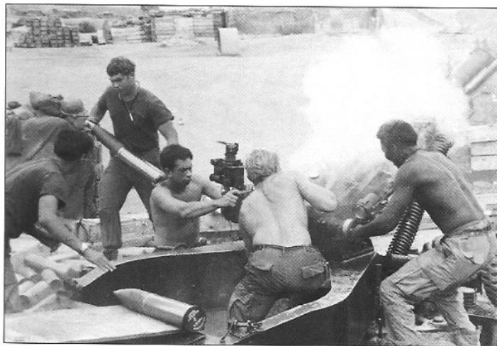
Rapid fire from an M102 105mm howitzer at FSB Charlie II (Quang Tri province) during Operation Dewey Canyon, March 26, 1971. Note the role of the single-unit trail in supporting the gun while the wheels are raised. The gunners are from Battery C, 6th Bn, 11th Artillery, (US National Archives)
