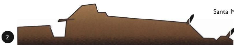
2. A cross-section of Fort Picurina's defences. Two rows of palisades protect the rear of the fort.
