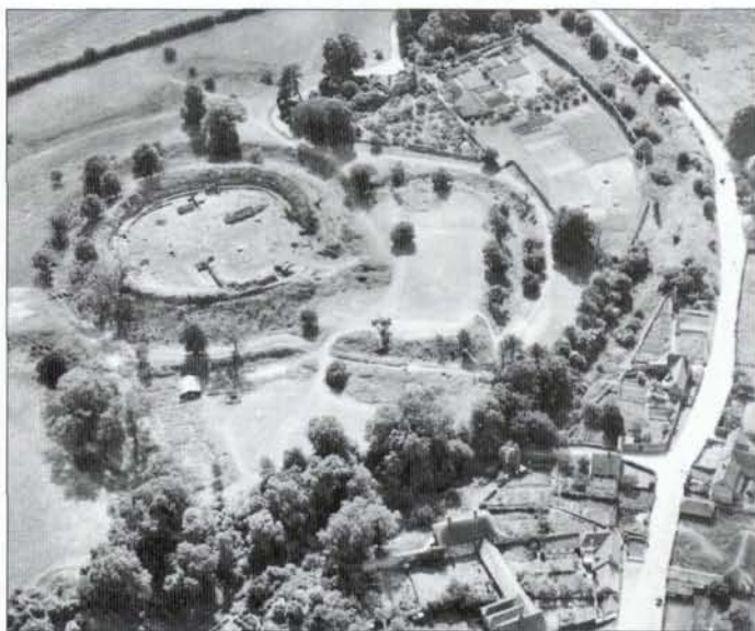
BELOW Basing House, Hampshire, a place described in a soldier's report of November 1643 as 'very strongly fortified ... strongly walled about with earth raised against the walls, of such a thickness, that it is able to de'd the greatest Cannon bullet'. (Photo: Cambridge University)
