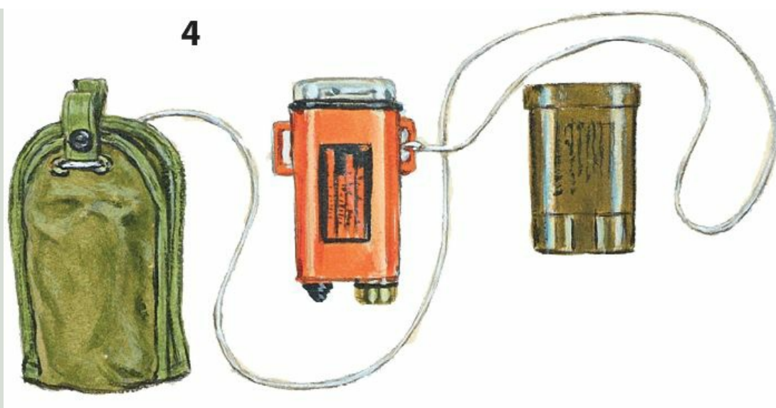
(4) SDU-5/E distress marker light (6230-067-5209 – “strobe light”), with its OD or sage-green nylon case, and the flash guard that was slipped over the body for stowage. It used a BA-1574/U battery.
