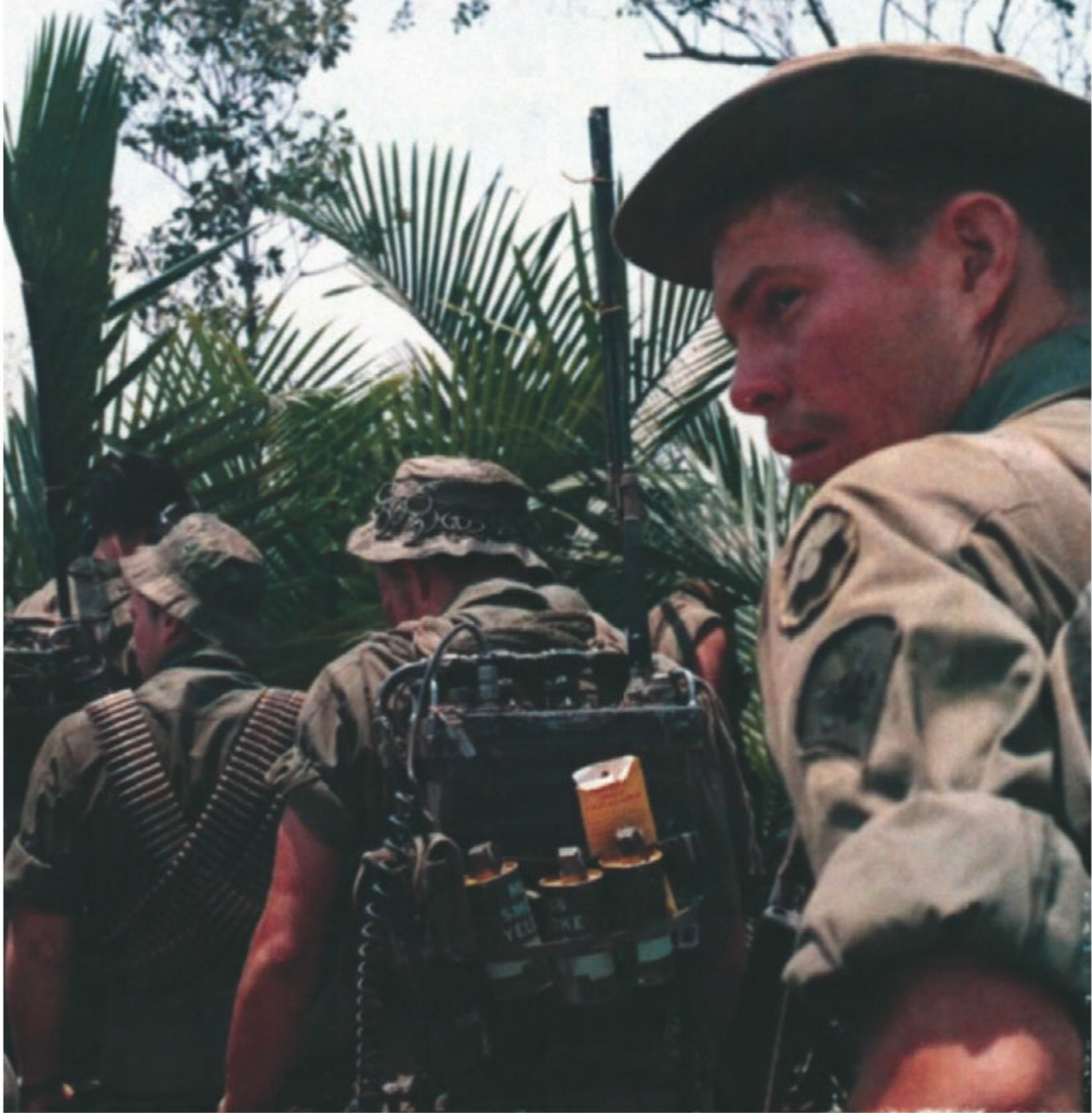
A 9th Inf Div radio-telephone operator (RTO) carries his AN/PRC-25 on the aluminum frame of a lightweight rucksack. Note that the long collapsible “whip” or “fishing pole” antenna is broken down into a bundle of sections linked by stretch cord, with the antenna’s base piece attached to the radio. This indicates that the unit is operating at some distance from the battalion firebase; at shorter ranges the 3ft “tape antenna” would be used. On the radio’s securing straps are three M18 yellow smoke grenades, and an orange envelope which holds pipe cleaners for cleaning the M16A1 rifle. (Tom Laemlein/Armor Plate Press)
