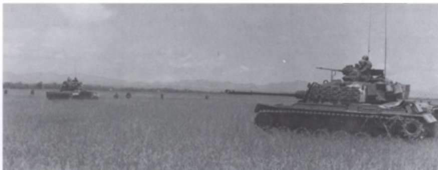
Only three Army and two Marine tank battalions operated in Vietnam, but they were not the only units to possess tanks – some of the armored cavalry squadrons also had some. Here M48A3 tanks mounting 90mm main guns cover infantry as they cross a broad, open area.
