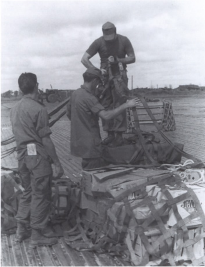
Many firebases and other installations could only be supplied by helicopter. Here rations are being rigged in cargo nets to be sling-loaded beneath CH-47 Chinooks.
