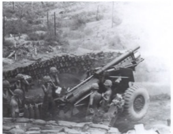
A 155mm M114A1 howitzer in full recoil. The steel tubes in the revetment wall are expended and earth-filled containers for propellant bags.
