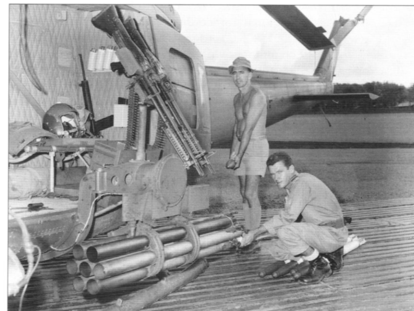
1969: publicity shot of a UH-1D 'Bushranger' gunship of No.9 Sqn RAAF being armed. The XM158 launcher pod for 7x 2.75in rockets, and a pair of M21 'Miniguns', made up the M16 armament system typically fitted to gunship Hueys. Above are 'twin sixties' in their stripped-down aircraft configuration, minus handguards but with added empty case defectors; the large storage bins held long continuous belts with many hundred rounds of 7.62mm ammunition. On the gunner's seat can be seen an AFH-1 flight helmet and aircrew body armour; an SLR – cut down in SAS fashion and with a 30-rd magazine – is stowed as a personal weapon. Wall bins hold further magazines and smoke grenades. The pilot wears RAAF rank and the RAAF's national title on the shoulder strap of his Australian flying suit.
