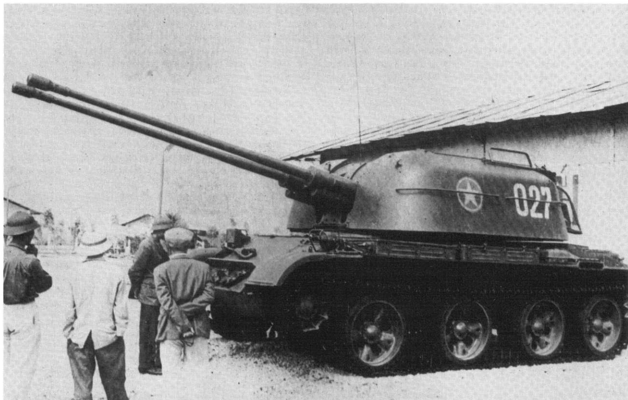
ZSU-57 self-propelled anti-aircraft gun on display in Hanoi, early 1970s. (Photo via F.C. Brown)
