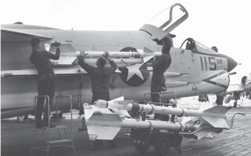
Ordnance personnel load AIM-9B Sidewinders on a VF-51 F-8E aboard Ticonderoga in February 1964, six months before the Gulf of Tonkin Incident. (US Navy)
