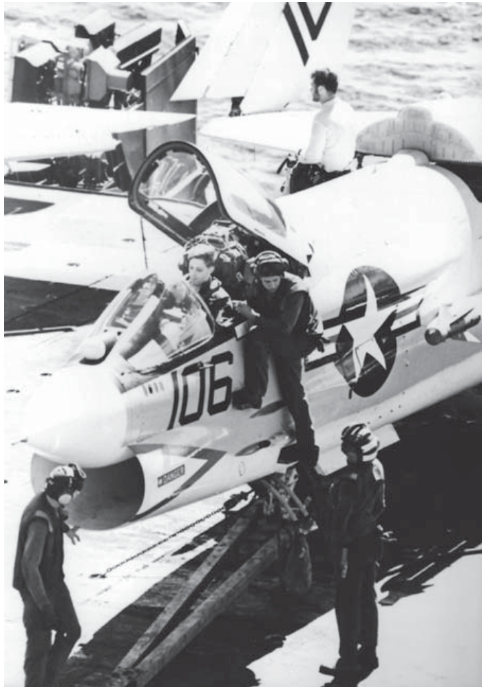
Lt(jg) Henry Livingston of VF-211 goes through his pre-start checks before launching from Hancock in 1972. His F-8J is armed with two Sidewinders, as well as the Crusader's internal 20mm cannon. (via Henry Livingston)
