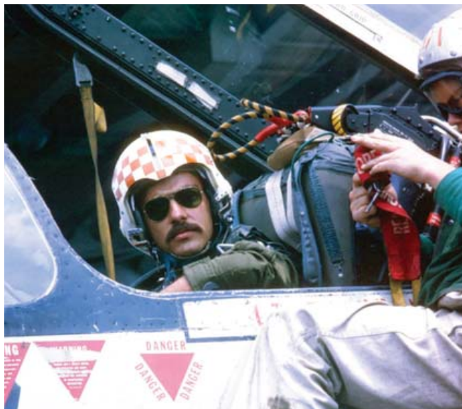
Lt Jerry Tucker of VF-211 prepares for a mission on Hancock ’s flightdeck in 1972. The plane captain (right) has pulled the safety pins from the F-8’s ejection seat, which is now armed. (John Stewart)
