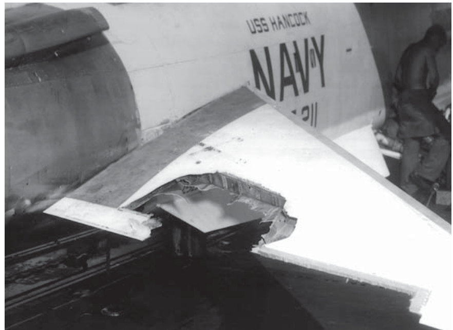
The extent of the flak damage inflicted on Vampatella's Crusader on June 21, 1966 is evident. Shortly after being hit by AAA Vampatella downed his MiG, thus proving the F-8's ruggedness. (US Navy)
