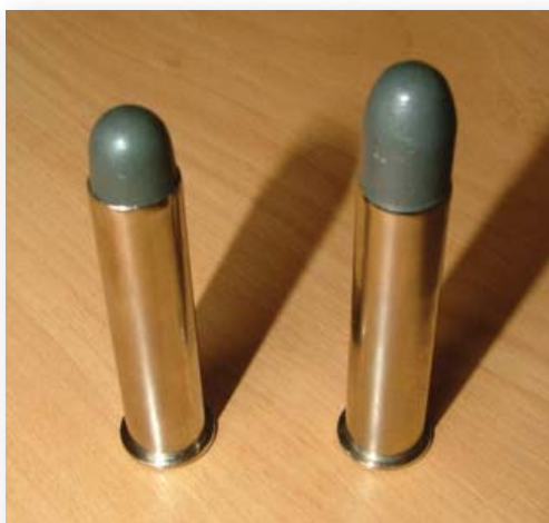
Replica Springfield 45/55 carbine bullet (left) and Springfield 45/70 rifle round (right). Both could be used by a carbine or rifle but the difference in size, evident in this photograph, meant that a rifle round loaded into a carbine would have a vicious recoil. (Author's photo)
