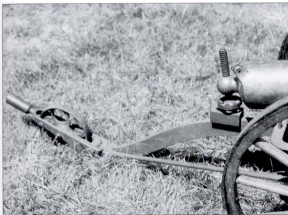
Detail of the elevating screw and wheel at the end of the carriage of the 12-pdr. Dahlgren boat howitzer. (George Lomas Collection)
