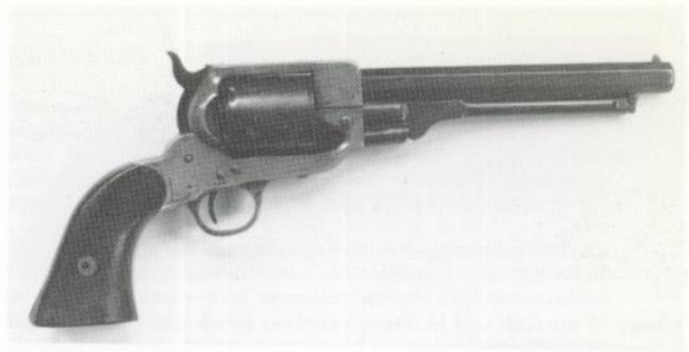
The Spiller & Burr revolver, with its brass frame and iron cylinder, hammer and barrel. This revolver sometimes came with a detachable shoulder stock. (Russ Pritchard)
