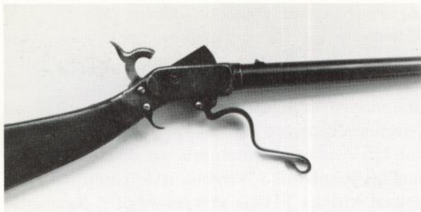
The Southern-made 'Perry' or 'Maynard' carbine. Brass-framed, it is 40 ins. long, with a 21½ in. barrel, and is of 0.52 in. calibre. It was probably made by N. T. Read of Danville, Virginia. (Russ Pritchard)
