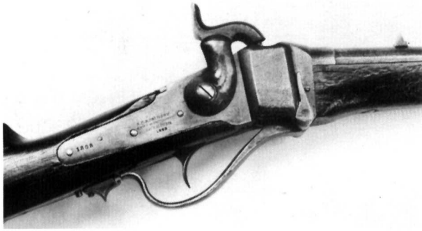
Detail of the lock of a Confederate-made, but fairly faithful copy of the Sharps carbine. The lock at the rear of the trigger guard was pulled back, the trigger guard/lever swung down and forward, and the breech block dropped, opening the chamber for the loading of a single round. (Russ Pritchard Collection)
