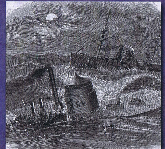
Best-suited for river combat the low freeboard and heavy turret of the Monitor made her highly unseaworthy in rough waters. As a result she foundered and sank while being towed south by USS Rhode Island during a heavy storm in the Atlantic off Cape Hatteras on December 31, 1862. Sixteen of 62 crewmen were lost in the storm. Based on descriptions by survivors, this engraving was published in Harper's Weekly on January 24, 1863. [Author's collection]
