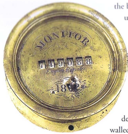
The engine register of the Monitor was recovered from the wreck site off Cape Hatteras, North Carolina, in 2001 and is one of only two artifacts recovered from the wreck bearing the name of the vessel so far. Small metal disks seen in the six small apertures slowly clicked over to show the engineer how many hours the ship's engine had been working for. [Courtesy of The Mariners' Museum]
