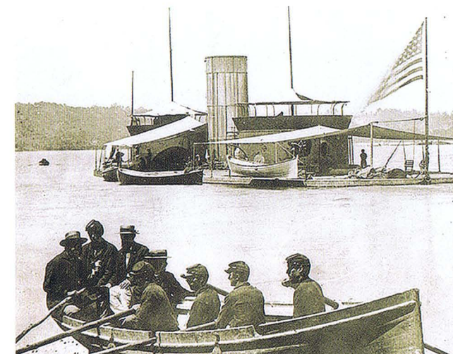
The first double-turreted monitor, the USS Onondaga , was photographed in the James River, Virginia, circa 1864/65. Note the awnings over the turrets and deck in an attempt to reduce the impact of hot weather on the vessel and crew. A detachment of Marines man the row boat in the foreground. [Naval Historical Foundation photo NH 60210]
