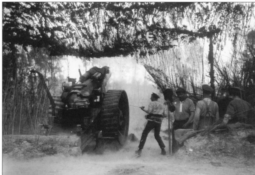
An 8in howitzer at the moment of firing. The gunner has just pulled the lanyard attached to the breech and the weapon is recoiling as the 200lb (91kg) high-explosive shell heads for the target. Note that the weapon is under a camouflage net, although the dust and smoke of firing would be difficult to hide. (IWM Q569)
