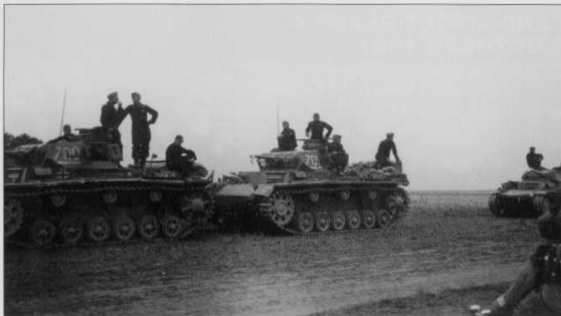
German PzKpfw II and PzKpfw tanks in an assembly area during the early phase of Operation Typhoon. These PzKpfw III tanks are still armed with the 37mm gun, rather than the better 50mm gun. (Nik Cornish)
