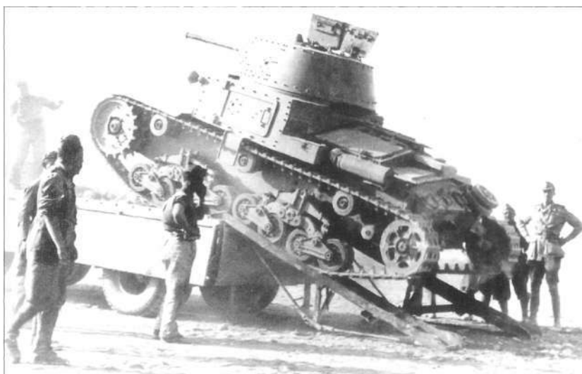
An Italian M13/40 tank being unloaded from a transporter. The tank was slow, uncomfortable and under-powered, but still served as the basic armoured vehicle in all of the Italian armoured units. Its 47mm gun, however, was accurate and its armour-piercing capability was superior to the British Crusader and Valentine tanks which were armed with the 2-pdr gun. (Ufficio Storico Esercito Rome)
