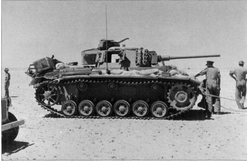
Captured Panzer III with the long-barrel 50mm gun being inspected by British troops. (IWM E16567)
