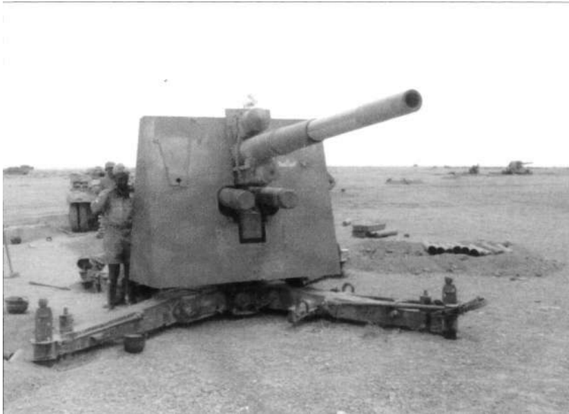
A battery of 88mm flak guns being used in an anti-tank role. The very high silhouette of the gun made it vulnerable to high-explosive counter-battery fire. (Bundesarchiv 1011-443-1574-24)
