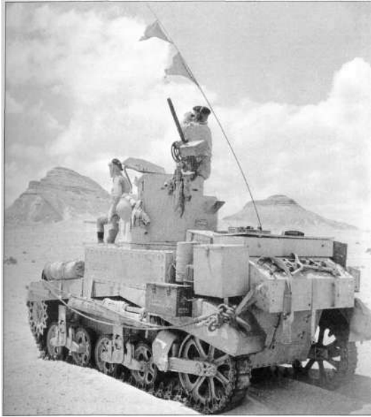
Early model American Stuart light tank in British service with riveted hull. The tank is from 7th Armoured Division and its crew are looking towards the high ground of Qaret el Himeimat. (IWME16095)
