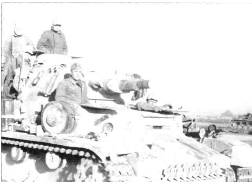
Panzer IV with short-barrel 75mm gun from 8th Panzer Regiment of 15th Panzer Division. Its triangular divisional sign can be seen to the right of the driver's slit. (Bundesarchiv 1011-439-1276-12)
