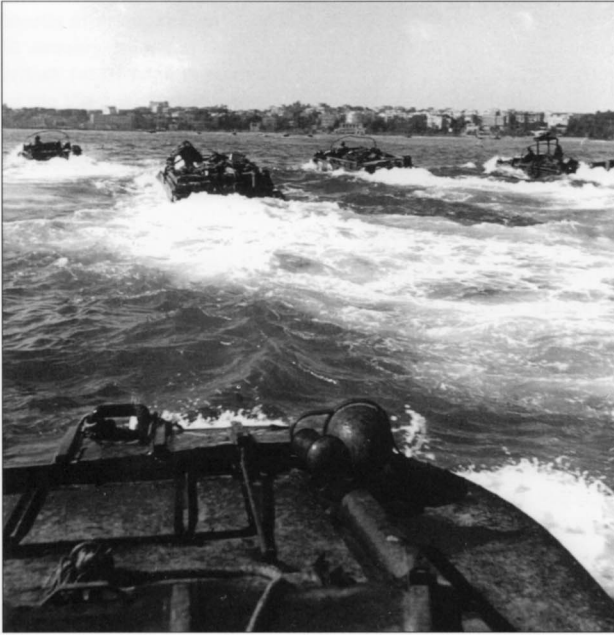
DUKW amphibious trucks head to the beach at Anzio on 22 January 1944. The DUKWs were the Allied secret weapon in the Mediterranean theater, able to deliver supplies to beachheads even if no port facilities were available. (NARA)
