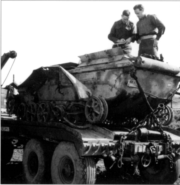
One of the innovations deployed against the Anzio bridgehead were the Borgward B.IV remote control demolition vehicles serving with Panzer Abt. (Fkl) 301. These carried a large high explosive charge that was dropped off against the target, and then the vehicle was remotely controlled back to safety before the charge detonated. These vehicles did not prove very effective at Anzio and this example is being examined by British officers on 20 April 1944. (NARA)
