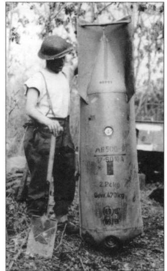
The Luftwaffe was very active over the Anzio beachhead, and a common weapon used against Allied troops was the AB500-1, a cluster bomb containing 37 SD-10 smaller submunitions. This is the empty case after the payload was dispensed. (NARA)
