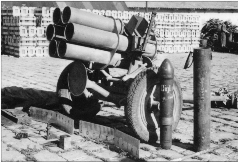
The 150mm Nebelwerfer multiple rocket launcher was dubbed the "Screamin' Meemie" due to the frightening sound of its rockets. A rocket is seen here alongside the launcher as well as its transport tube. (NARA)
