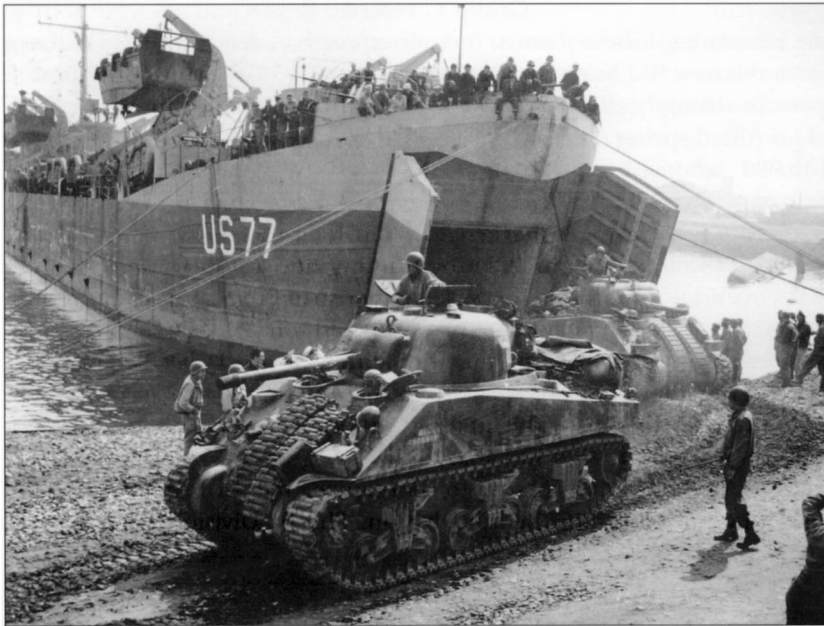
In anticipation of Operation Buffalo, the remainder of the 1st Armored Division was moved into the beachhead to assist in the assault and here some of the division's M4 tanks are seen unloading from an LST. (NARA)
