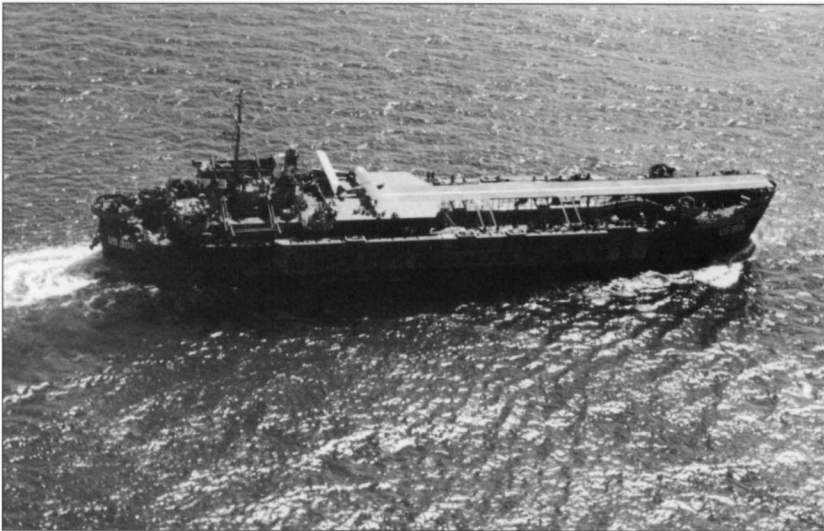
One of the more intriguing Allied innovations used at Anzio was the addition of a flight deck to LSTs by 3rd Division engineers. This permitted L-4 observation aircraft to fly artillery observation missions from offshore when airbases were not available in the beachhead. (NARA)
