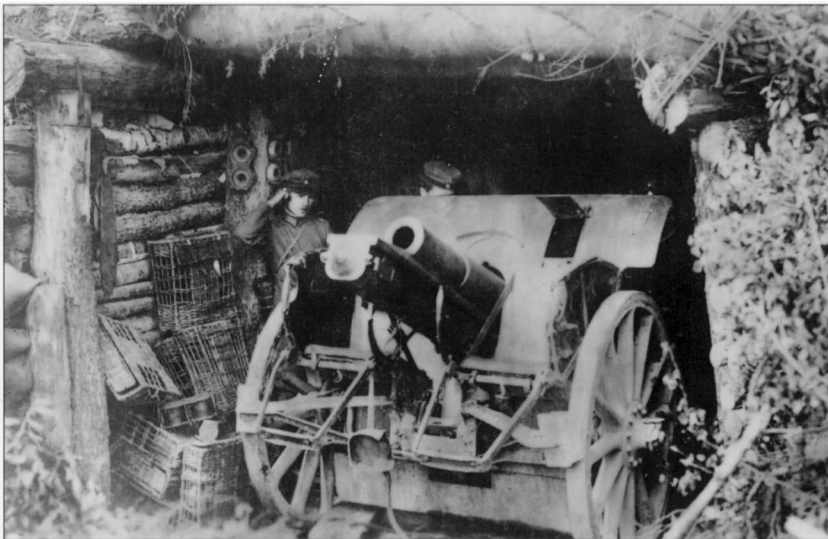
A German 10.5cm light field howitzer in an emplacement. This workhorse of the German field artillery could hurl a 33lb shell up to 6,000m. Each infantry division was equipped with 12. (IWM, Q23721)
