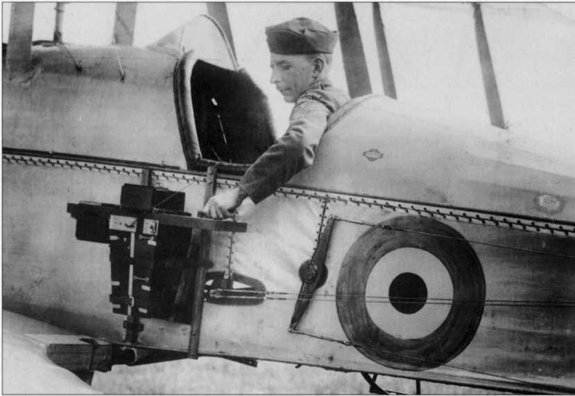
A camera fitted to a BE2c aircraft. Do not be misled by the improvised mount and primitive equipment. They produced imagery of superb fidelity. Altitude and orientation in flight were also carefully logged to assist survey. (IWM, Q33850)
