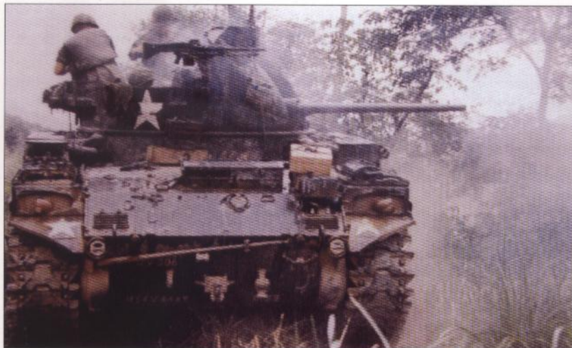
The twin 40mm M42A1 Duster self-propelled anti-aircraft vehicle also mounted a 7.62mm M60 machine gun for close-in defense. The twin Bofors guns pumped out 240 rounds per minute of high-explosive tracer and armor-piercing tracer, the latter able to defeat a PT-76 tank. The Army provided two of these deadly weapons for Khe Sanh.
