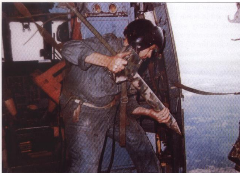
Airborne-delivered sensors played a key role in the defense of Khe Sanh, here an Air-Delivered Seismic Intrusion Detector (ADSID). There were several versions, and could detect the vibration of troops moving (seismic) or be activated by the sound of voices and movement (acoustic). Monitoring stations picked up the signal, and the general area in which the sensor had been planted was saturated by artillery and air strikes.
