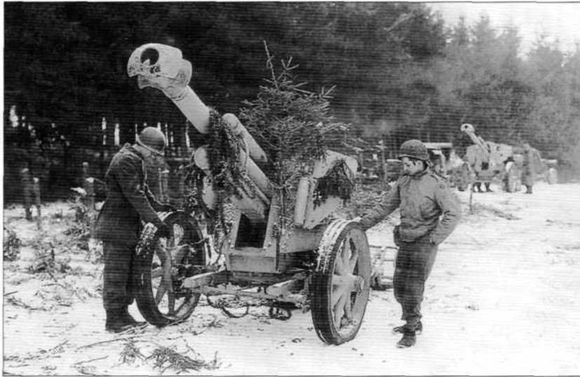
The workhorse of the German field artillery was the 105mm field howitzer like these that were captured by the 35th Division near Lutrebois on 17 January 1945. This is the improved leFH 18/40, which used the lighter carriage of the PaK 40 anti-tank gun. (NARA)
