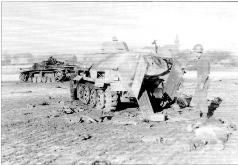
A Kampfgruppe of the Führer Grenadier Brigade attacked Patton's 80th Division in Heiderscheid on Christmas Eve and amongst its losses were the StuG III to the left and this SdKfz 251 half-track, one of the rare SdKfz 251/17 variants with a turreted 2cm autocannon. (NARA)
