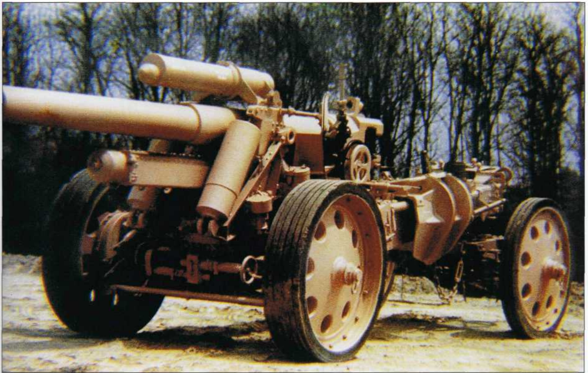
Heavy firepower for German artillery was provided by the schwere Feldhaubitze 18 15cm. These served in a heavy artillery battalion in German infantry divisions. (MHI)
