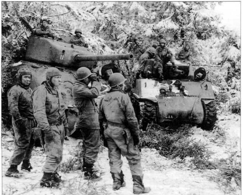
A tank patrol of the 3rd Armored Division scans for signs of the 116th Panzer Division near Houfallize on 23 December. The tank to the left is an M4A1 (76mm) while the one to the right is an M4A3E2 assault tank. (NARA)
