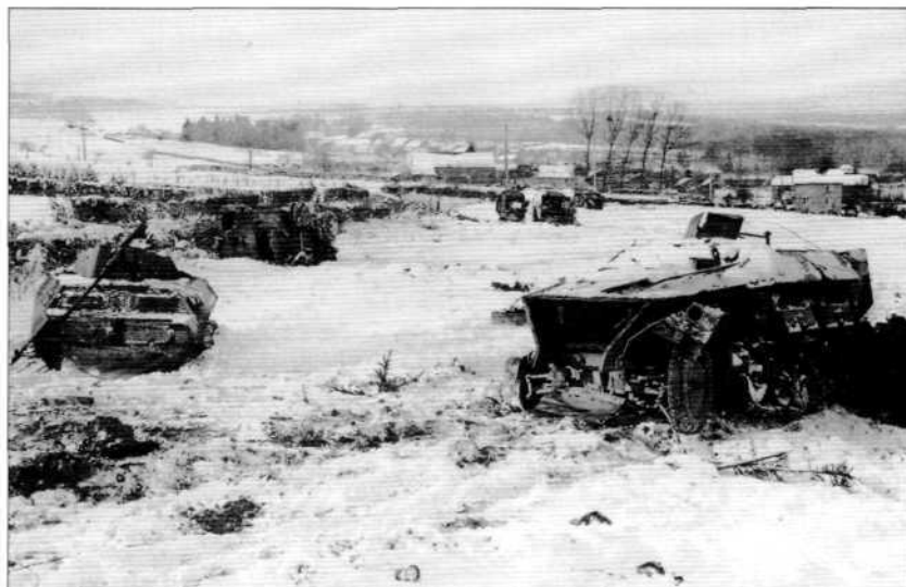
The fields around Amonines are littered with the wrecks of SdKfz 250 half-tracks of the 116th Panzer Division, destroyed during an encounter with Task Force Orr of the 3rd Armored Division. The vehicle to the left is an unusual variant with a 2cm cannon.
