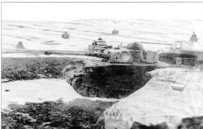
German Panzer regiments in the Ardennes were of mixed composition, including the PzKpfw IV as seen here in the center, and the later Panther Ausf. G seen above and to the right. In the foreground is a SdKfz 251/9 (7.5cm), an assault gun version of the standard German armored half-track used to provide fire support in Panzergrenadier units. (USAOM-APG)
