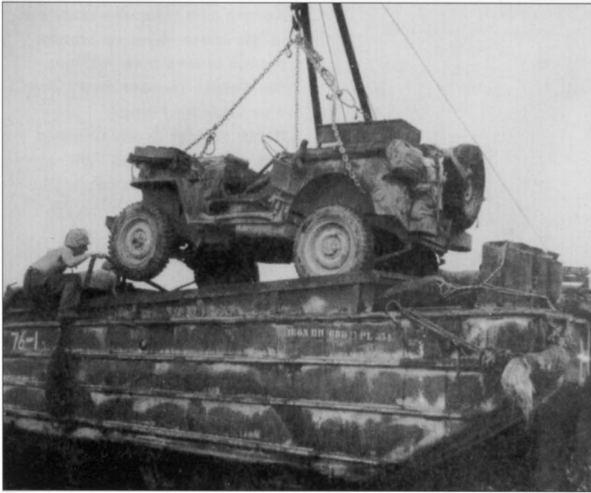
Although used earlier, the 2½-ton DUKW-353 amphibian truck (“Duck”) was employed in large numbers; some 50 in each in two Army and two Marine amphibian truck companies. Some Ducks were fitted with A-frame hoists for cargo unloading once ashore. Able to carry 5,000lbs of cargo, they were mainly used to haul in light artillery and ammunition.
