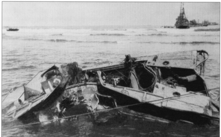
The remains of an LVT(2) destroyed by a horned anti-boat mine on "White 2". Mines also destroyed two other amtracs. Although 100 mines were found on the beach, most had deteriorated or were unarmed. The amtrac's bow is to the left. The mine detonated beneath the driver's compartment.
