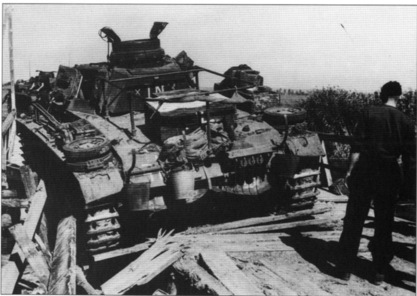
Panzerbefehlswagen Ausf. E or H of 36th Panzer Regiment staff proves too heavy for wooden bridge in rural Ukraine during battle for Kiev. German engineers repaired the bridge the same day so the regiment could continue its advance.
