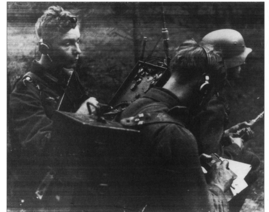
German Pack Wireless Type d2 for company-battalion-regiment communications. Radios gave the Germans an advantage in command and control. During all of Barbarossa they captured only 149 radios from the Soviets, who relied excessively on the telegraph.
