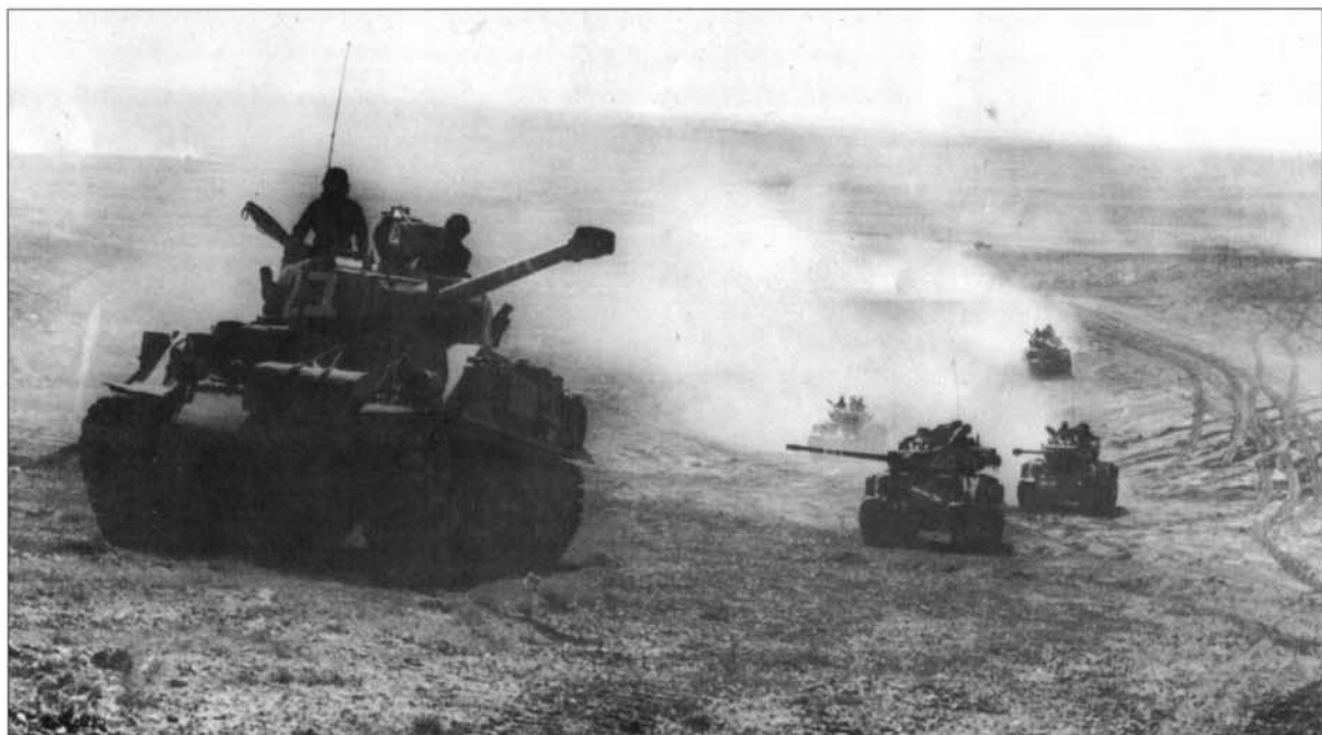
This column of Israeli 'Super Shermans' rolls across terrain typical of that in the area of operations in the Sinai Desert. Rolling sand dunes kick up the ever-present clouds of dust to parch throats and clog engine filters; the latter had to be cleaned repeatedly to avoid damage to the engines.
