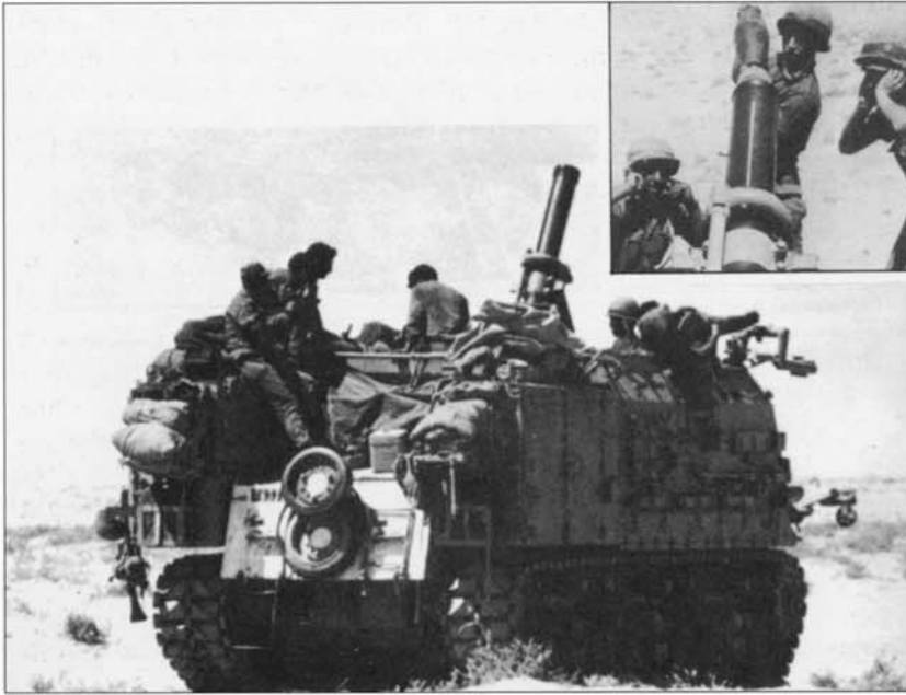
A Soltam 160mm self-propelled heavy mortar is prepared for action in the Sinai Desert. Another Israeli self-propelled artillery weapon based on the Sherman M4A3E8 chassis, the breech-loaded heavy mortar is capable of accurate, indirect fire out to a range of 10,000m (10,900yds) with a total of 56 mortar rounds carried on board the vehicle.
