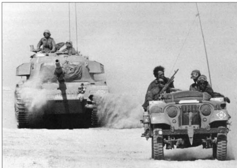
An M38 Jeep of an armoured battalion's reconnaissance company leads an Upgraded Centurion across the desert sands towards the Suez Canal. It was just such a Jeep-mounted reconnaissance unit or 'Sayeret' that found the gap between the Egyptian Second and Third Armies that allowed Operation Gazelle to be launched.
