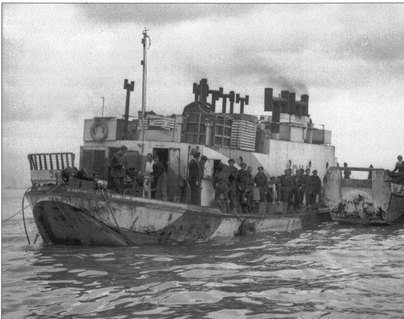
Crews from infantry landing craft come alongside a landing barge kitchen (LBK). This converted Thames barge was equipped to provide hot meals for ferry craft crews. On D-Day alone, this barge served over 1,000 meals to the sailors and marines who operated the exposed assault landing craft. The inclusion of LBKs in the invasion fleet demonstrates the amount of attention to detail that was required during the planning of operation Neptune. (Imperial War Museum, A24017)
