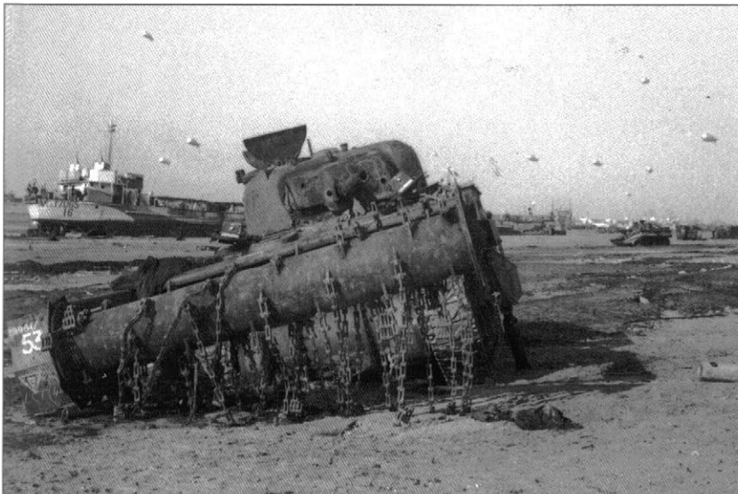
Sherman Crab flail tank of the Westminster Dragoons, knocked out on Gold Beach during the assault phase. The metal chains on the revolving drum at the front of the tank were designed to beat a path through minefields, detonating the charges as it went. (Imperial War Museum, B5141)
